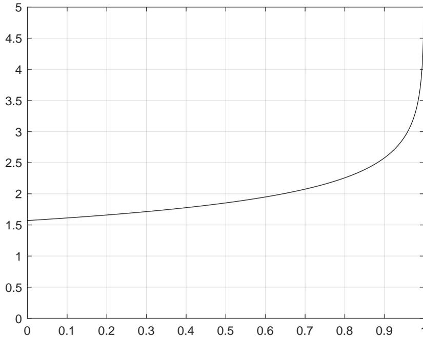
Figure 3: Complete elliptic integral of the first kind.
